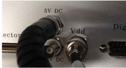
Figure 9: Agilent E3630A power supply plugged into 5V DC of WHISPER Box. Note the orientation of the GND tab of the BNC to banana plug cable. Reversing the polarity of the power supply might damage the hardware.
