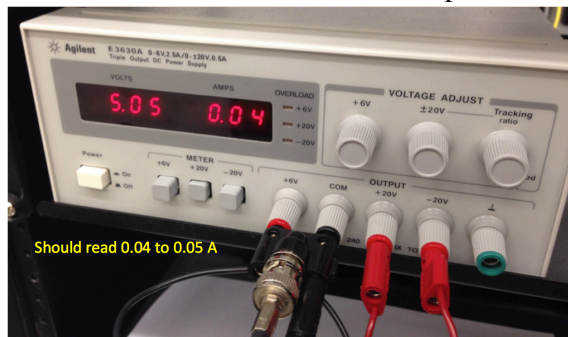
Figure 11: Agilent E3630A power supply when both powered with 5V & -5V DC
