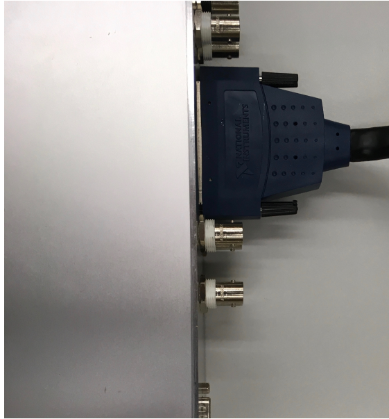
Figure 12: NI cable plugged into WHISPER Box
